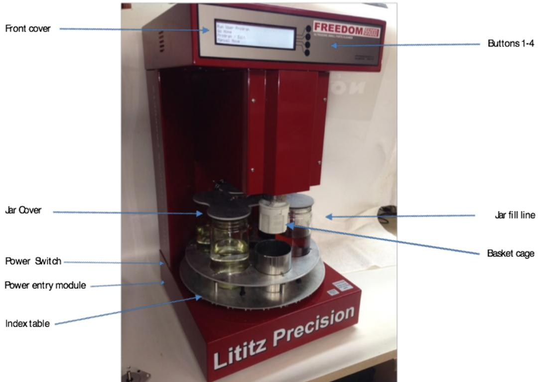
Place the Freedom on a level surface. Remove the packing material that is in and around the jar cover. Plug the supplied cord into the power entry on the left rear of the machine, and then into a grounded wall receptacle. The required voltage and current is listed on the rear of the machine. Turn on the machine using the switch located on the power entry module. The “Freedom” splash screen will appear for 5 seconds. To exit from this screen before five seconds, press any button.
