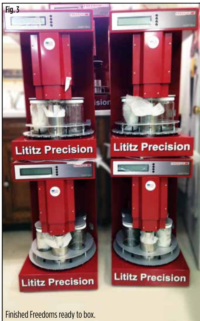
The most recent venture of Baer and LPP is the Freedom automatic cleaning machine, Figure 3. This new machine is the brand's most ambitious project yet. The Freedom consists of five stations for cleaning or rinsing, all with ultrasonic, and one drying station. There are 10 user-customizable programs with agitation strength and station time programmable at each station. Surprisingly, this was the most difficult part
