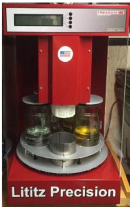
The two model FREEDOM cleaning machines, are both automatic and fully ultrasonic in all four or five jars. Made and assembled here in the U.S., the design and production is the brainchild of a watchmaker-engineer, John Baer, in Lititz, Pennsylvania, where the town is known for its horological expertise far away from any bustling metropolis.
