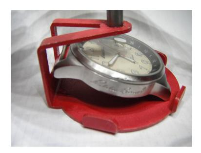
Place the watch holder assembly inside the jar and lower the watch into the water by lowering the lifting knob.
