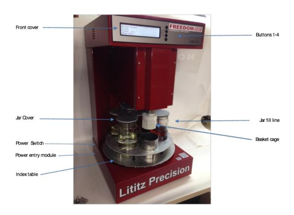
Place the Freedom on a level surface. Remove the packing material that is in and around the jar cover. Plug the supplied cord into the power entry on the left rear of the machine, and then into a grounded wall receptacle. The required voltage and current is listed on the rear of the machine. Turn on the machine using the switch located on the power entry module. The "Freedom" splash screen will appear for 5 seconds. To exit from this screen before five seconds, press any button.
